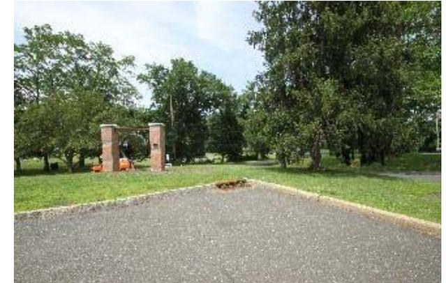
Parking spots south of the building can be replaced with porous asphalt to capture and infiltrate stormwater. A wide drive way east of the building can be de-paved or converted into pervious pavement. Additionally, a rain garden can be installed beside the parking lot to capture, treat and infiltrate runoff. A preliminary soil assessment suggests that soils have suitable drainage characteristics for green infrastructure.
