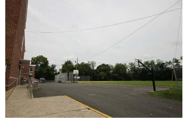
Parking spots and a basketball court can be replaced with pervious pavement to capture and infiltrate stormwater. Pedestrian walkways around the school can be replaced with pervious concrete to capture stormwater as well. A preliminary soil assessment suggests that more soil testing would be required before determining soil suitability for green infrastructure.
