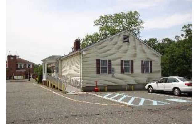
Stormwater is currently directed to existing rain barrels and catch basins throughout the site. The paved picnic area beside the building can be replaced with permeable pavers to capture and infiltrate stormwater. Parking spaces can be replaced with porous asphalt to capture and infiltrate runoff as well. A preliminary soil assessment suggests that soils have suitable drainage characteristics for green infrastructure.
