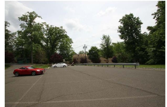
Runoff from the parking lot currently drains toward the road. Parking spaces can be replaced with porous asphalt to capture and infiltrate stormwater. A rain garden can also capture, treat and infiltrate runoff on the site. A preliminary soil assessment suggests that more soil testing would be required before determining soil suitability for green infrastructure.
